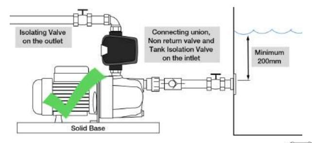
In this example the water level is higher than the pump inlet but the water cannot flow freely into the pump.
